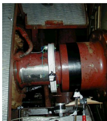
Figure 1. Strain gauges mounted on the propeller shaft
